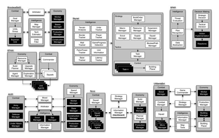
Fig. 3. Architecture of 7 StarCraft bots obtained by analyzing their source code. Modules with black background sent commands directly to StarCraft, dashed arrows represent data flow, and solid arrows represent control.
